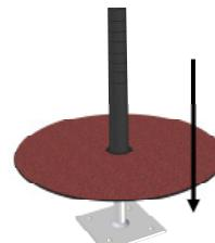
2. Cut the PP-moulding with a knife at one of the provided grooves. Then shrink the special shrinking tube by moderately heating from top to down (using a hot air blower or small, gentle flame) over the transition between LUX-top® anchor point or descent point and moulding (overlapping 50/50). Adhesive must visibly escape from the top edge of the shrinking tube.
