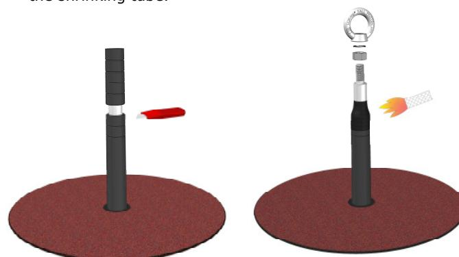
3. Using a small welding torch, work the whole bitumen flange into the roof waterproofing and all round the plate.
