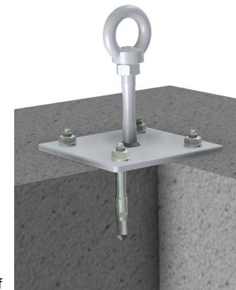
1. Use a Ø 10 mm drill bit to drill 75 mm deep holes from the top edge of the base plate.
