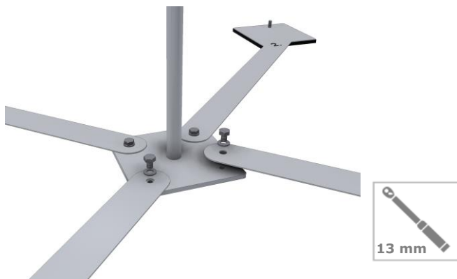
Fig. 3: Bolting the feet
