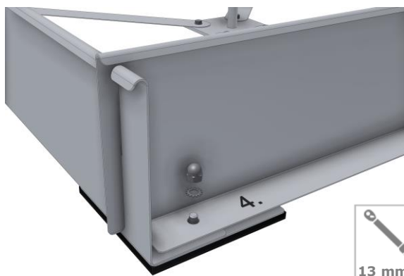
Fig. 6: Fixing the edging
